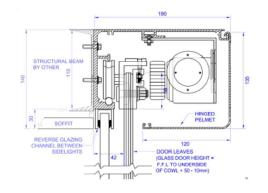
Diagram indicates concealed integrated installation for frameless glass door (right) and Aluminium framed installation to entry framing (left).
